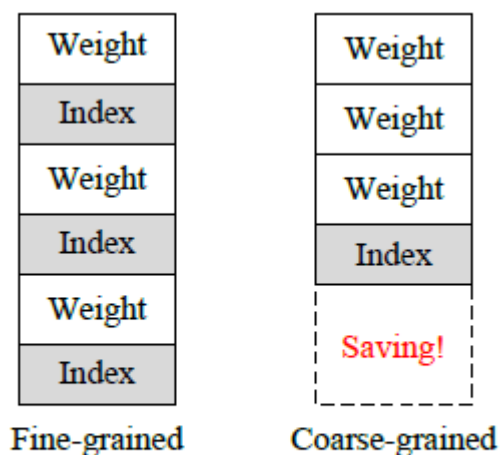
Figure 5: Illustration of index saving.
