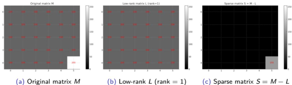
Figure 2: Matrix decomposition  $M = L + S$  with rank-1 background: original data  $M$ , low-rank background  $L$ , and sparse anomaly  $S$ .
