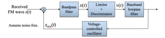
Denote  $s(t) = \cos(2\pi f_c t + \phi(t))$ , and let  $s_{\text{vco}}(f) = 2\cos(2\pi f_{\text{vco}}t + \phi_{\text{vco}}(t))$  with  $\phi_{\text{vco}}(t) = \alpha\phi(t)$ . Show that
