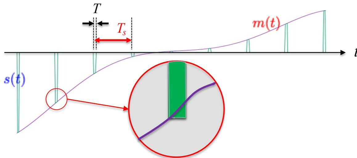
*Notably, the top of each pulse is maintained **flat**. So, this is PAM, not natural-sampling for which the message signal is directly multiplied by a periodic train of rectangular pulses.*
