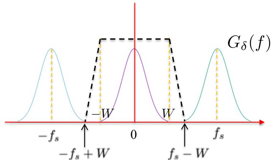
Signal spectrum with bandwidth  $W$
