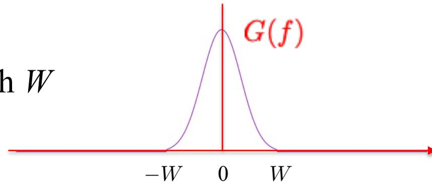
Signal spectrum after sampling with  $f_s > 2W$
