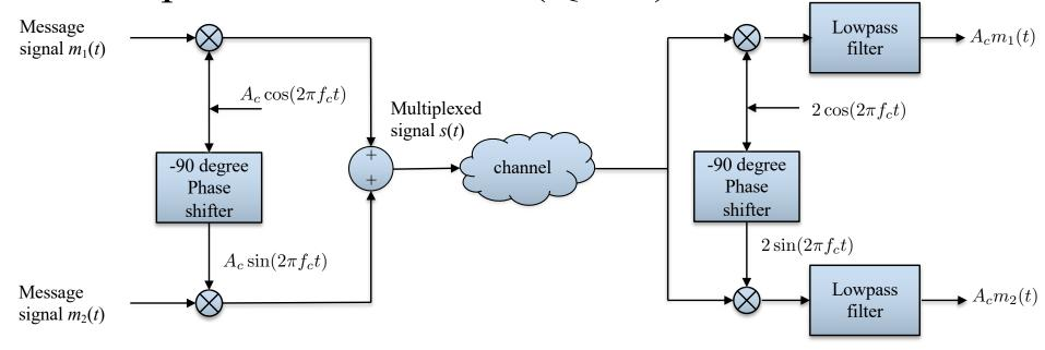
Synchronization is critical in QAM, which is often achieved by a separate low-power pilot tone outside the passband of the modulated signal.
