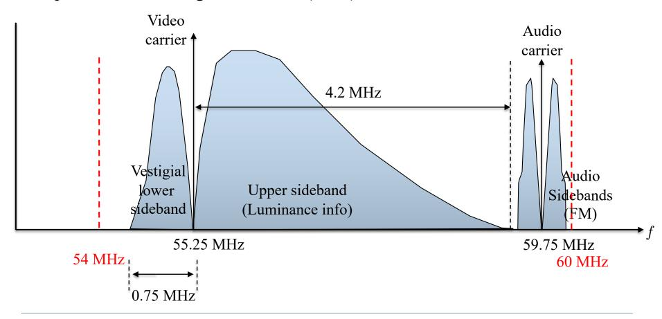
☐ As the transmission signal is not quite VSB modulated, the receiver needs to "re-shape" the received signal before feeding it to a VSB demodulator.
