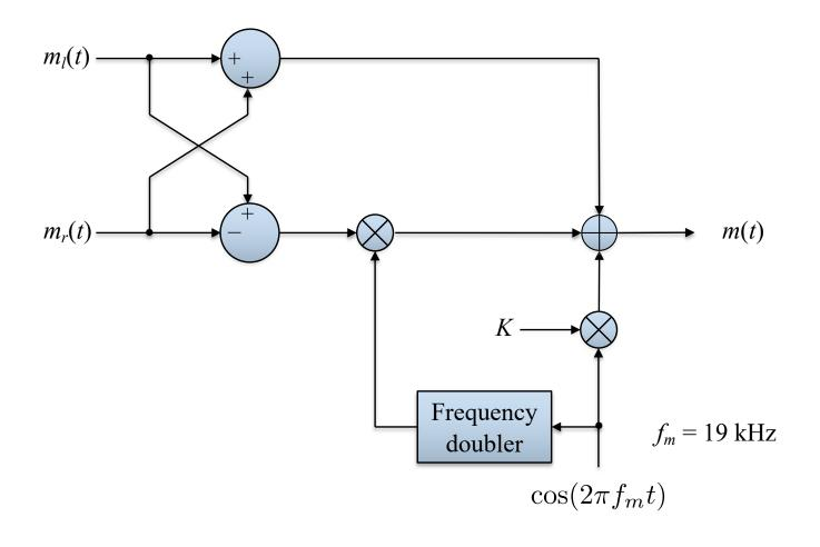
$$m(t) = \underbrace{\left[m_l(t) + m_r(t)\right]}_{\text{For mo nophonic reception}} + \left[m_l(t) - m_r(t)\right] \cos(4\pi f_m t) + \underbrace{K\cos(2\pi f_m t)}_{\text{For coherent detection}}$$
