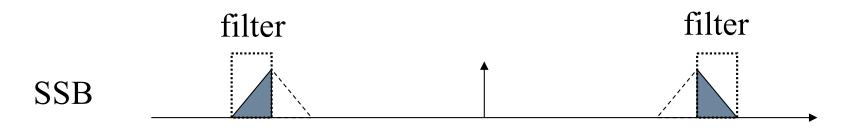
☐ For the generation of a SSB modulated signal to be possible, the message spectrum must have an *energy gap* centered at the origin.
