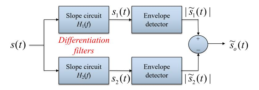
$$H_{1}(f) = \begin{cases} j2\pi a \left( f - f_{c} + \frac{B_{T}}{2} \right), & |f - f_{c}| \leq \frac{B_{T}}{2} \\ j2\pi a \left( f + f_{c} - \frac{B_{T}}{2} \right), & |f + f_{c}| \leq \frac{B_{T}}{2} \\ 0, & \text{elsewhere} \end{cases}$$
