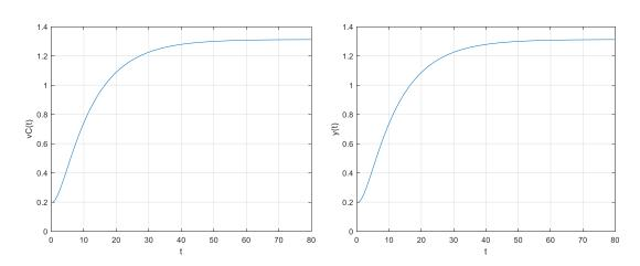
The simulation results of  $v_c(t)$  based on (2-73) and y(t) based on (2-74) are shown in the above figures, left and right respectively. It is easy to observe that both are the same as expected.
