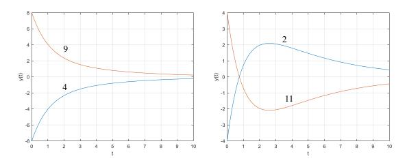
Besides, any curve bounded by these two straight lines has the property y(t)>0 or y(t)<0, such as the solution of Curve 4 and 9. On the other hand, any curve outside these two straight lines, such as Curve 2 and 11, has the property that y(t) first reaches its maximum or minimum at y'=0 and then converges to 0.
