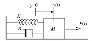
In engineering, most of the systems are constructed by mechanical components such as dampers and springs. The simplest one is shown in the figure, called the mass-damper-spring system or MBK system in brief, where M is the mass of the moving object, B is the damping coefficient of the damper and K is the stiffness of the spring. Let F(t) be an extra force exerted on the object at time t and assume y(t) is the
