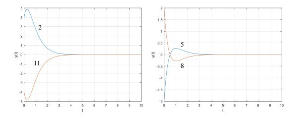
The resulted portrait of y(t) is shown in the phase plane, where Curve 6 and Curve 7 belong to the same straight line with slop  $\lambda = -2$ . All the other curves have the property that y(t) first reaches its maximum or minimum at y' = 0 and then converges to 0, such as y(t) of Curve 2 and 11 and y(t) of Curve 5 and 8.
