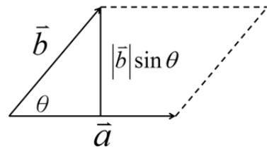
$$\Rightarrow |\bar{a} \times \bar{b}| = |\bar{a}| |\bar{b}| \sin \theta = \text{the parallelogram determined by } \bar{a} \text{ and } \bar{b}.$$
